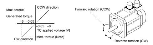
Generated torque limit values will vary about 5% relative to the voltage depending on products. Generated torque may vary at the voltage of -0.05V to +0.05V.
